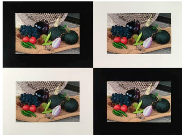
Figure 12. An example image of the CIPA chart as it was captured during the test with the given setup. The analysis is performed in the image center.
