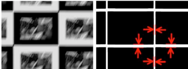
Figure 3. Analysis of motion blur in CIPA DC-X011 left : An image of the test chart, captured with a device under test while it was shaken (cropped) right : The measurement of the motion blur, based on black and white corners in the chart. The image shows a binary representation of a filtered version of the original image.
