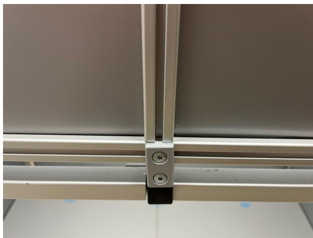
Figure 10- 1 Attaching the lightSTUDIO AW head with the mount
