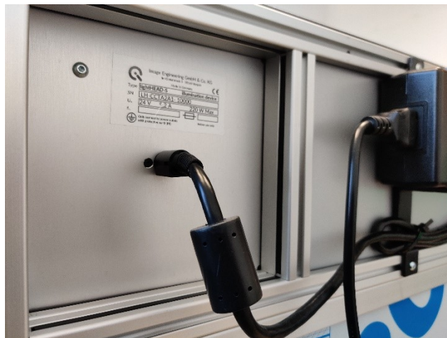
Figure 6-2 Connecting the lightSTUDIO AW head to the power supply unit
