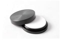
The white reference RESTAN based on PTFE (Polytetrafluoroethylene) diffusely reflects more than 98% of light in the area between 300nm and 1700nm. This means the reflection level is higher and more uniform especially at longer wavelength than the reflectance of barium sulfate (BaSO4).
