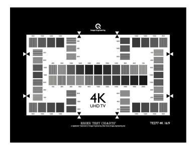
The TE277 is designed to measure and describe the frequency response of an electronic 4K (UHD TV) camera.
