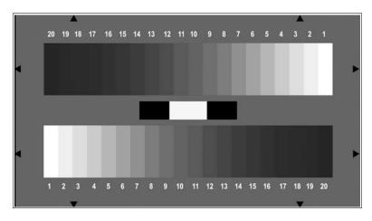
The TE259 is designed to check the dynamic range of broadcasting cameras on a waveform monitor. Two 20-step graduated counter current gray scale are arranged on a gray background, the gray scale is NOT graduated logarithmically nor linear! Densities are measured relative to the brightest patch.
