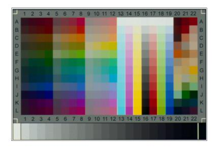
The TE258 is designed to characterise slide/print scanners.
