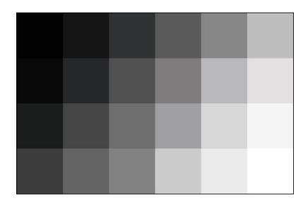
The TE240 D is designed to determine the dynamic range and the scanner opto electronic conversion function (OECF). The OECF describes how the scanner transforms luminance values of the object into digital code values in the digital image. The OECF is typically measured from a gray scale.
